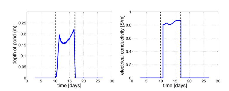
Level of pond water (far left) reveals when to expect onsets of infiltration and drainage (vertical black dashed lines)
